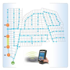
iTracking analytics immediately discover that micro basin 1C, comprised of adjacent manholes 1B - 1C, is contributing 75% of the I&I within all of mini basin 1.
